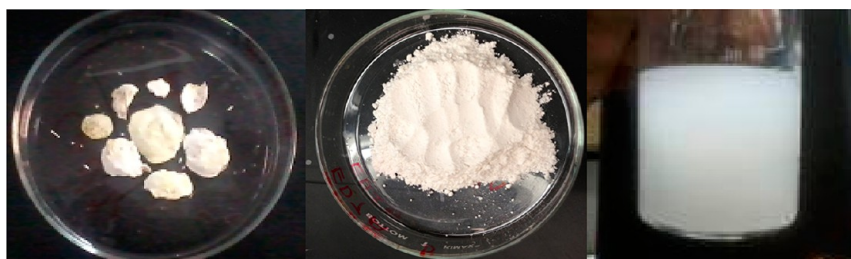
Figure 1. Photographic images of water-washed cellulose nanocrystals (left), alcohol-washed cellulose nanocrystals (center), and alcohol-washed cellulose nanocrystals dispersed in water (right).
